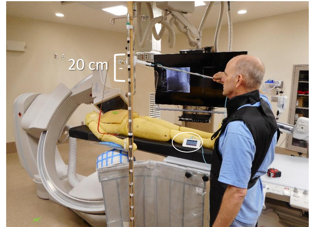
RaySafe X2 Scatter Radiation Meter Measurements 20-200 cm From the Floor, in 20 cm Intervals
