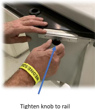
Figure 15: Place the Head Flex Shield on the head rail and secure it by tightening knobs
