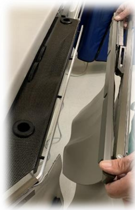
Figure 14: Attaching the Side Flex Shields to the rails on the patient's right side of the EggNest XR™ system
